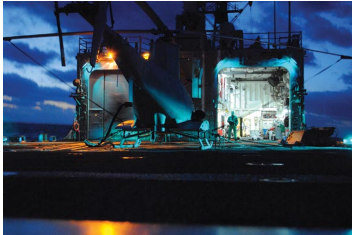
The Northrop Grumman-built MQ-8B Fire Scout VUAS conducting shipboard flights from the USS Halyburton (FFG-40) to verify that its communications link with the ship is functioning properly. (Photo Courtesy of the U.S. Navy)
