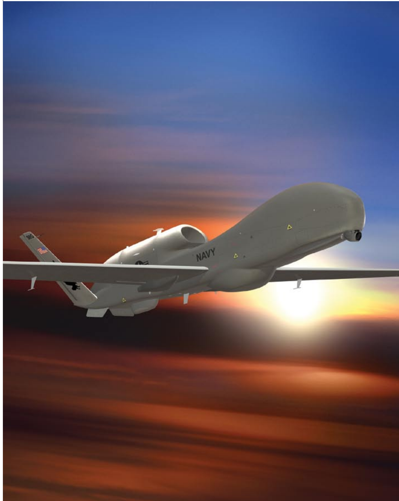
The United States Navy's MQ-4C Broad Area Maritime Surveillance (BAMS) Unmanned Aircraft System (UAS) program provides persistent maritime Intelligence, Surveillance, and Reconnaissance (ISR) data collection and dissemination capability to the Maritime Patrol and Reconnaissance Force (MPRF).
