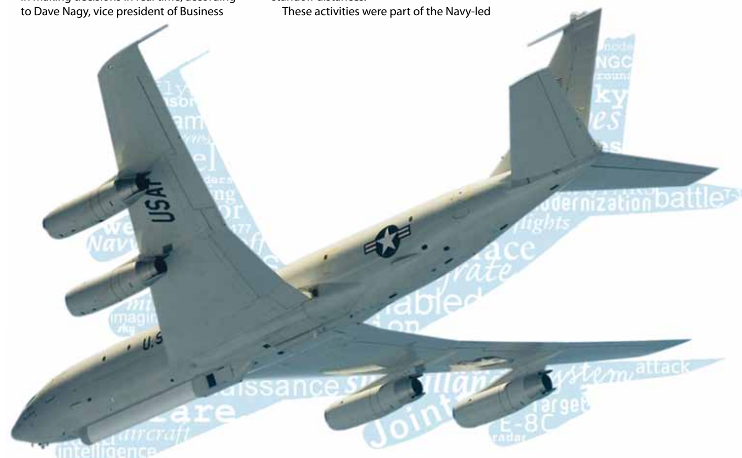
A Northrop Grumman E-8C Joint Surveillance Target Attack Radar System test-bed aircraft, with its new JT8D engine propulsion pod system, performs a multi-sensor demonstration with the APY-7 radar system and the multispectral sensor, MS-177, located immediately aft of the radar in the new keel beam accessory bay.
