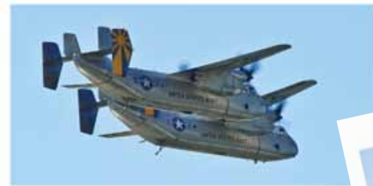
Two Grumman C-2A Greyhounds rumble along to pay tribute to the 100th anniversary of naval aviation. Developed from the Grumman E-2 Hawkeye, the C-2A Greyhound is a twin-engine cargo aircraft designed in 1966 to shuttle mail and supplies between U.S. Navy aircraft carriers.
