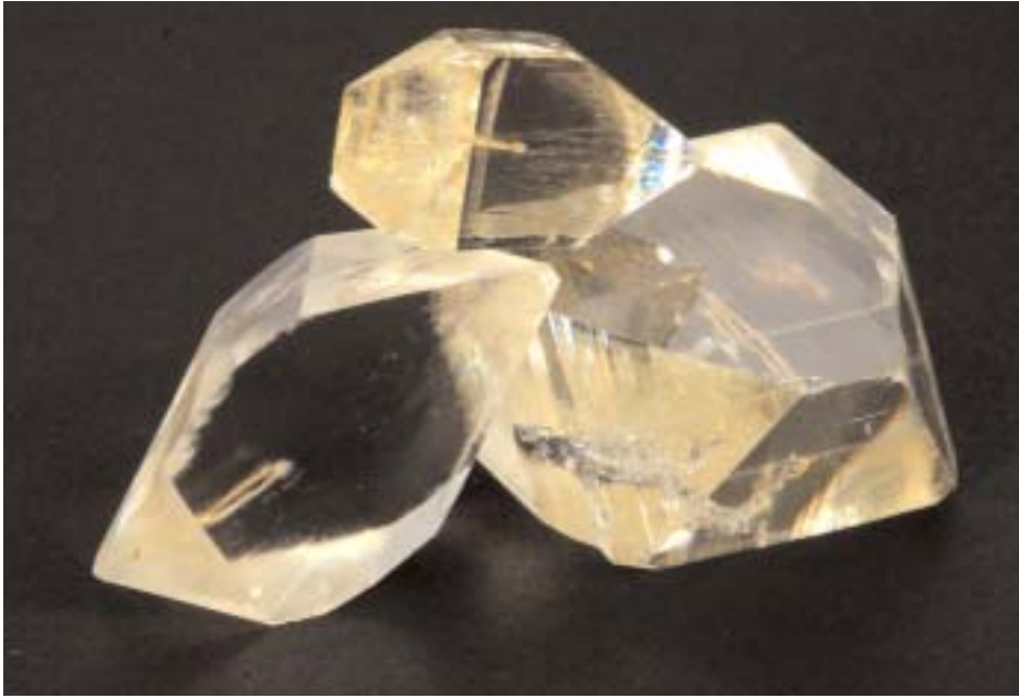
Hydrothermally-grown KTP crystals for the medical market
