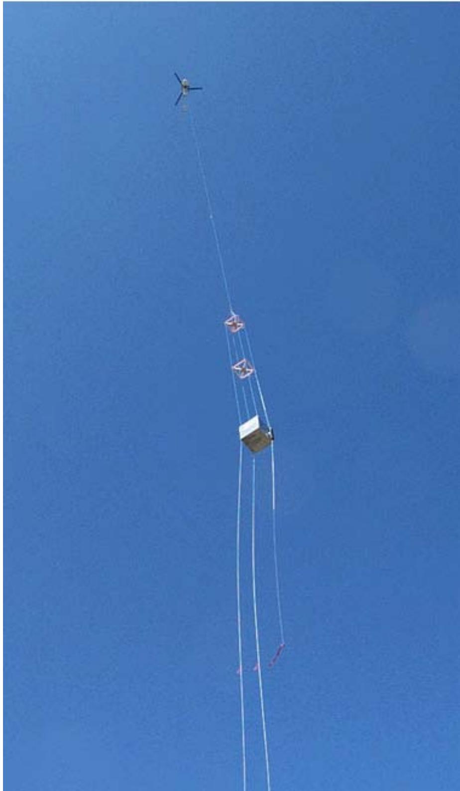
Figure 10. RF Test Equipment Suspended from Helicopter
