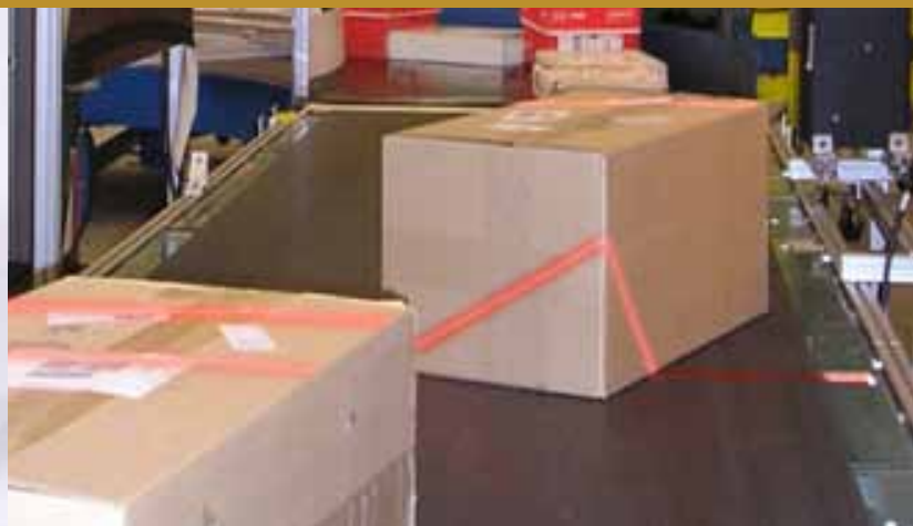
Boxes being counted, measured, and checked for their position, orientation and mail type by the AOA Xinetics measurement system.
